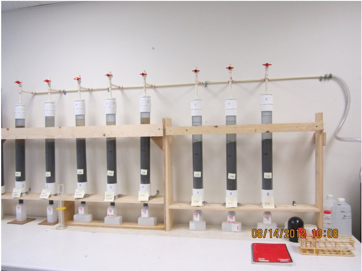
Figure 2. Otter Creek Column Leach Set Up (photo courtesy Energy Labs, Helena)
